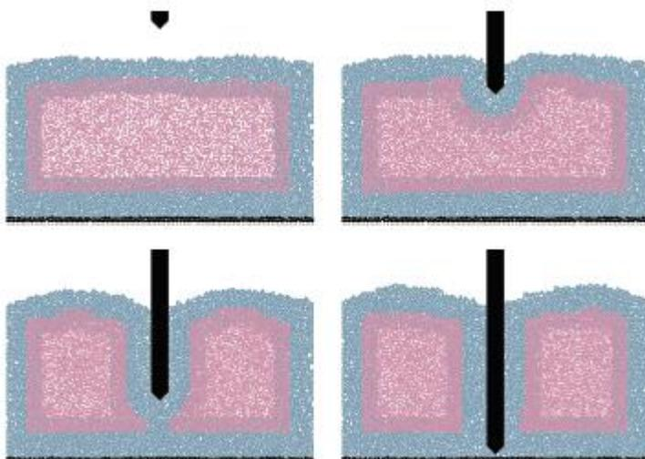
Insertion of cone penetrometer, from Yue et al. (2018)
