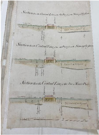
Sections of the river bed at 3rd, 4th and 6th piers of Tyne bridge, Newcastle, 1771 [Royal Society Smeaton drawings JS/4/67v]
