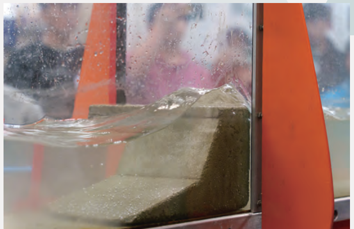
A seawall model undergoing wave load testing in the Water Resources Laboratory
